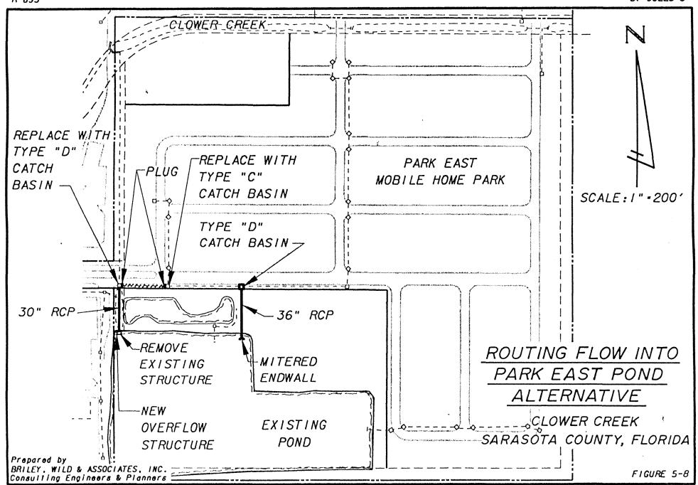
The re-routing of the storm sewers and the reconstruction of the pond with a littoral zone and a new overflow structure and discharge pipe is estimated to cost approximately \$30,000. Table 5-14 summarizes the costs incurred in this alternate.
