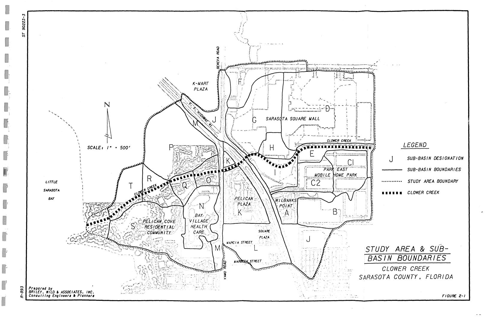
The upper 1,200-feet of the Creek is a V-shaped ditch approximately 8-feet deep with an average top width of 40-feet. This portion of the Creek is a fairly uniform natural channel overgrown with weeds and underbrush. This section of the Creek collects piped stormwater discharge from the east pond of the Sarasota Square Mall and a small portion of the Park East Mobile Home Park. Overland flow also enters the Creek from the south.
