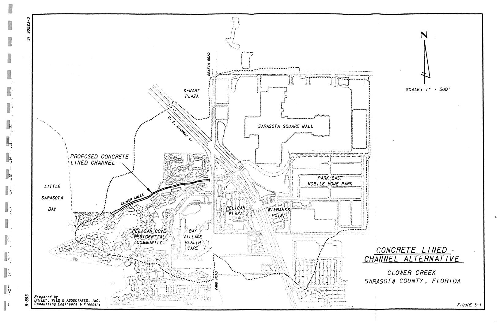
The disadvantages of this alternative include a very high capital cost. Another disadvantage of this alternative is that it offers no reduction in sediment inflows from upstream areas. A concrete lined channel would require removal of all natural vegetation. The existing biological community would be permanently impacted. This impact is unacceptable from an environmental view point and therefore, would require significant mitigation to offset the impact.
