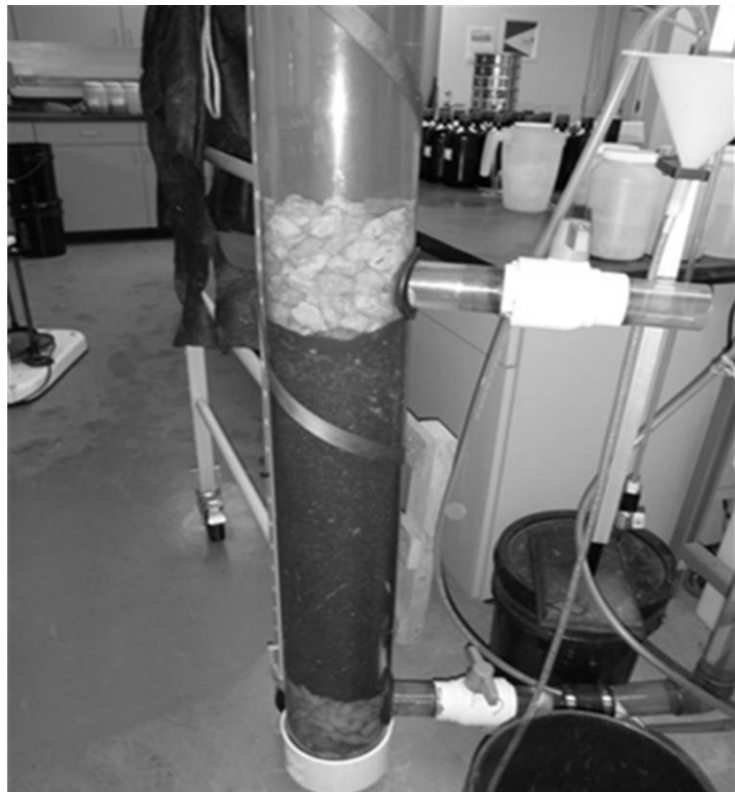
Figure 2.3 Media Bench Scale Column Testing of BLSS Water Source (UCF, 2009)
