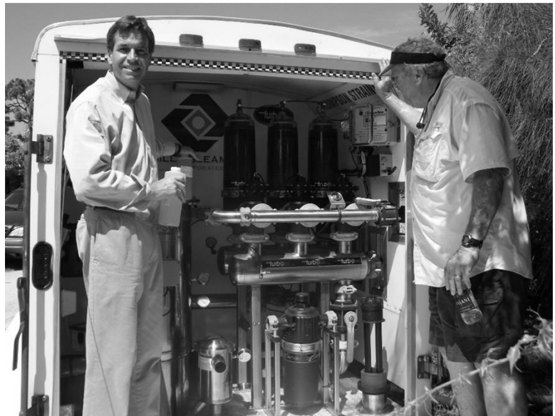
Figure 2.2 Briarwood Lakes Stormwater System Field Testing of Mechanical Disc Filtration System
