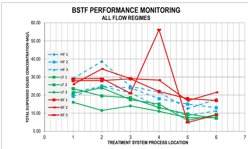
There is little if any demonstrated benefit in solids settling in the first solids settling basin (Location 2). Some limited solids settling effectiveness is demonstrated in the aerobic zone.
