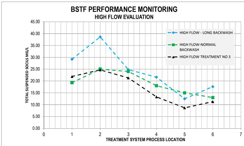
**2.2 TN Results:** The TN reduction from an HF operational protocol demonstrated effective settling and filtration capacity of organic solids to consistently reduce TN with high influent background concentrations (above 2 mg/l). It should be noted that lower TN influent concentrations (less than 1.5 mg/l) was linked to lower treatment effectiveness. It is possible that dilution effects of rainfall changes the environmental dynamics of treatment.
