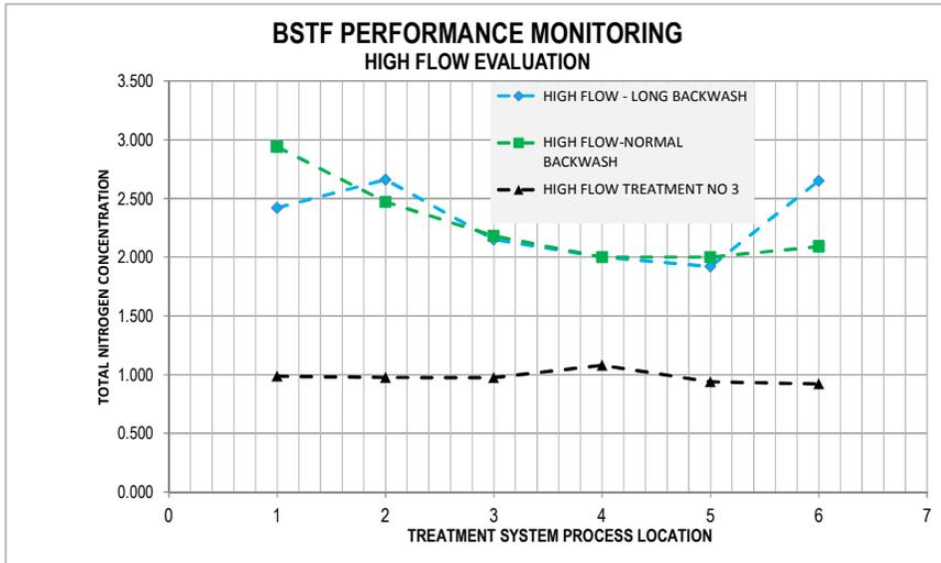
**2.3 TP Results:** The TP reduction potential from a HF operational protocol demonstrated less effective pollutant reductions through the aerobic zone but some removal was still noted through upflow filter processes. Note that the long backwash cycle appeared to negatively impact performance of the aerobic zone.
