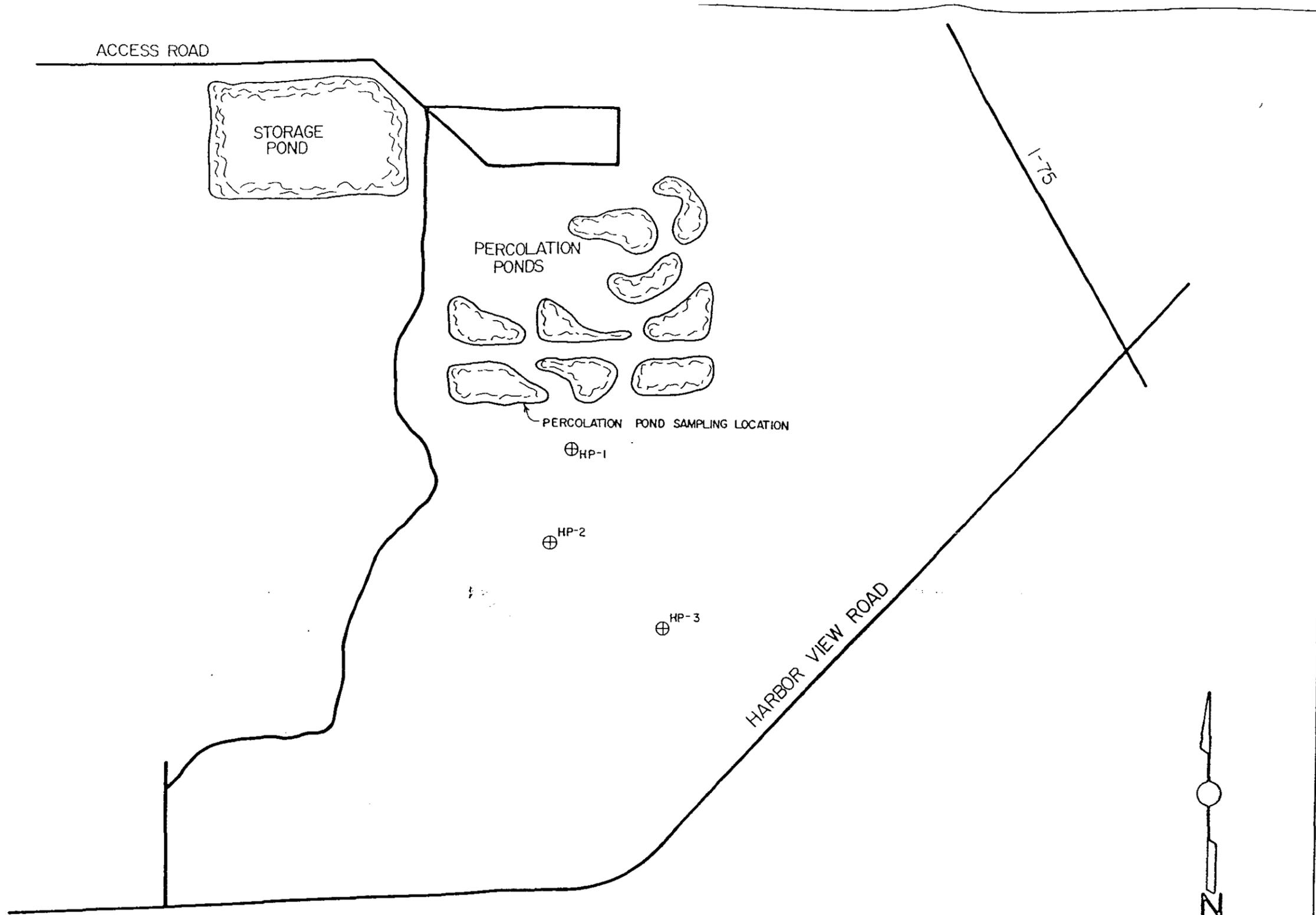
⊕ HP - PIEZOMETER AND HORIZONTAL PERMEABILITY TEST LOCATIONS
