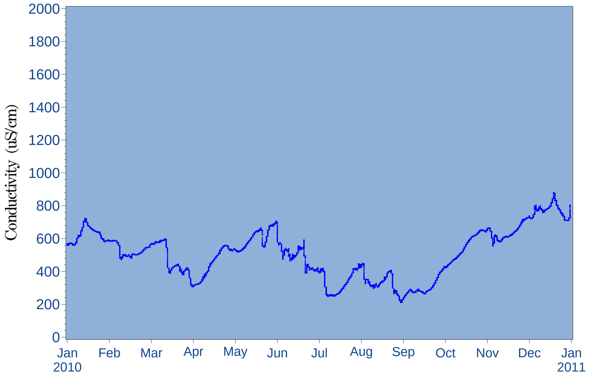
Figure 5.20 2010 Surface conductivity (15-min intervals) for Peace River fixed station at Peace River at Platt (Facility) - USGS gage 02297345 (River Kilometer=29.8)
