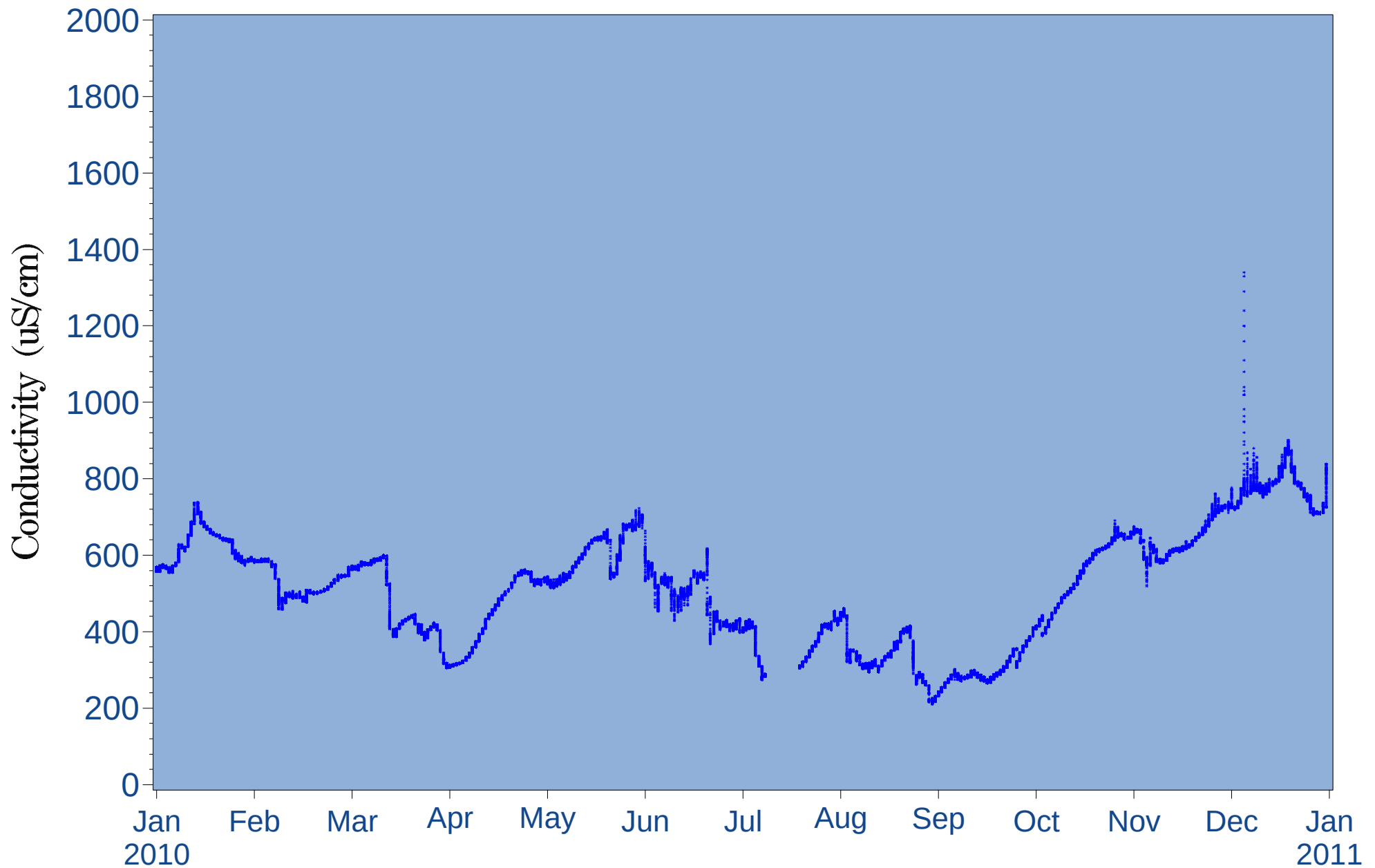
Figure 5.21 2010 Bottom conductivity (15-min intervals) for Peace River fixed station at Peace River at Platt (Facility) - USGS gage 02297345 (River Kilometer=29.8)
