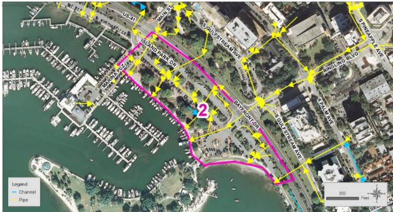
Figure 8-12 Aerial View of Site 2 (SWFWMD, 2010) with Sarasota County Stormwater Inventory
