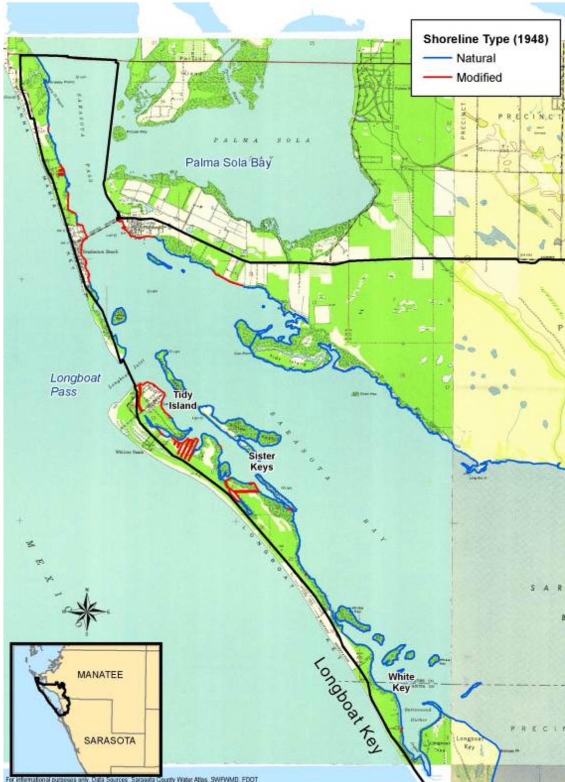
Figure 2-5 1948 Quad Map of Sarasota Bay with 1948 Hardened and Natural Shoreline Shown (North Area)
