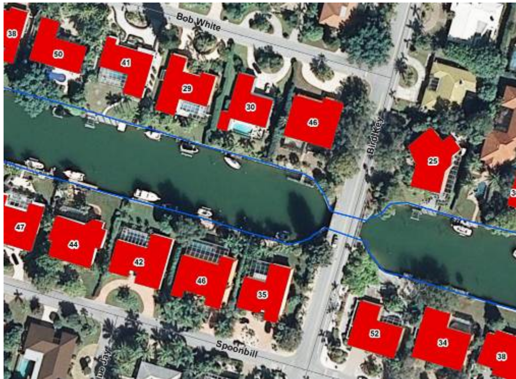
Figure 5-4 Digitized Home Footprints and Swimming Pools Which Are Not Included in Building Footprint (Note: Number in black denotes distance [feet] from edge of structure to watercourse.)
