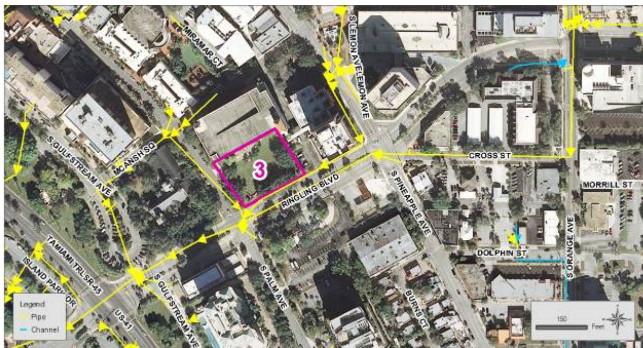
Figure 8-14 Aerial View of Site 3 (SWFWMD, 2010) with Sarasota County Stormwater Inventory
