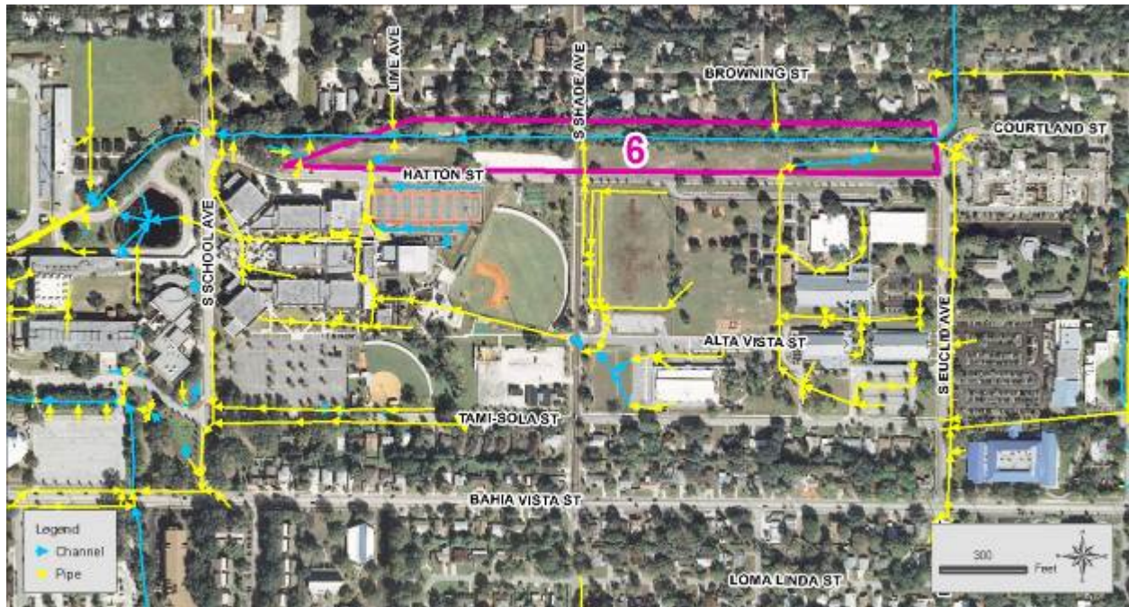
Figure 8-26 Aerial View of Site 6 (SWFWMD, 2010) with Sarasota County Stormwater Inventory
