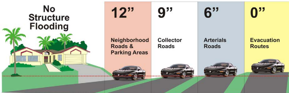
Figure 4-1 Acceptable Flooding for a 100-Year Storm
