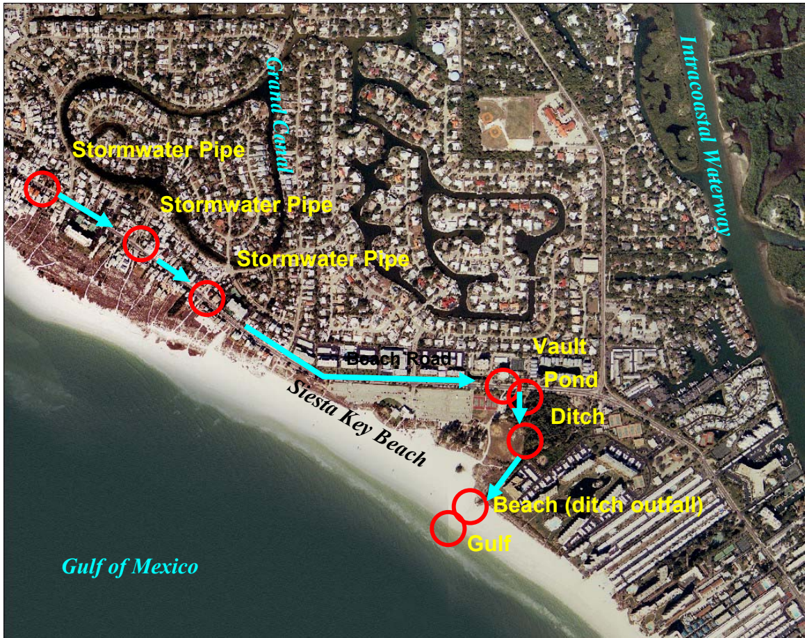
Figure 5. Sampling locations within the stormwater system draining to Siesta Key Beach (light blue arrows indicate general direction of stormwater flow).
